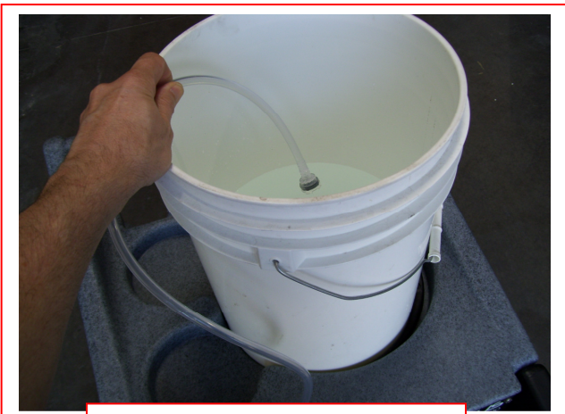
Place Chemical Feed Hose into Rinse Solution
