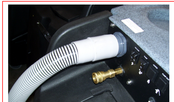
Vacuum connection with standard barb and vinyl cuff
