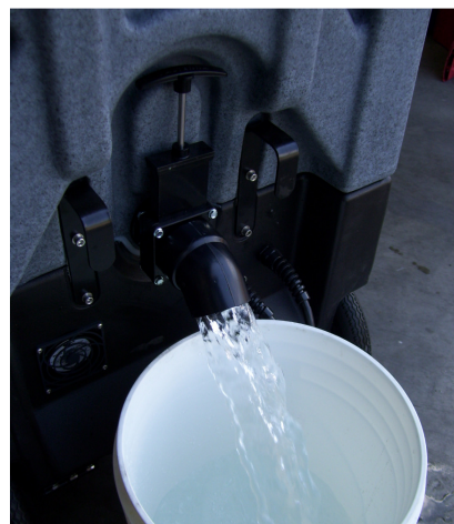
Drain water from Recovery Tank
